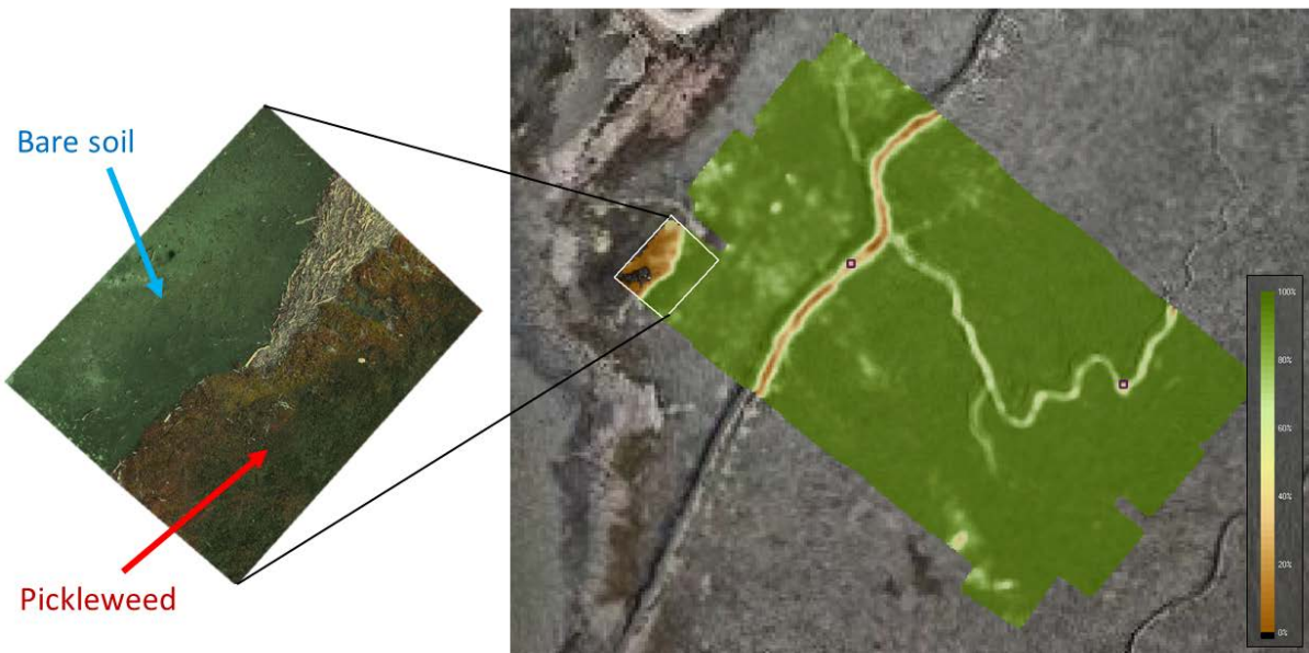
Figure 8. Vegetation index: Multispectral imagery captured using the ACMAD unmanned air system (UAS) at Ecology Marsh. (Right image) Proportion of the landscape with vegetation is shown as green, with less vegetated land surface shown as yellow to brown. (Left image) Image captured from the UAS camera showing bare soil (blue arrow) and pickleweed (red arrow).
