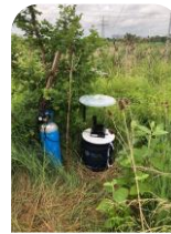
Automated mosquito counting and remote reporting trap
